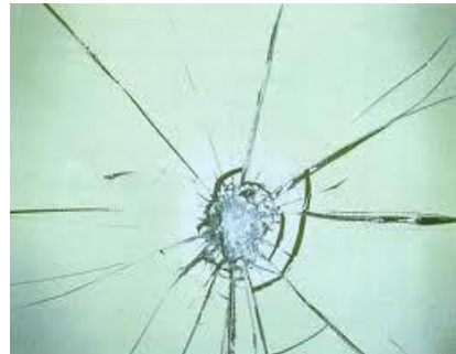
• Laminated Glass shatter pattern
